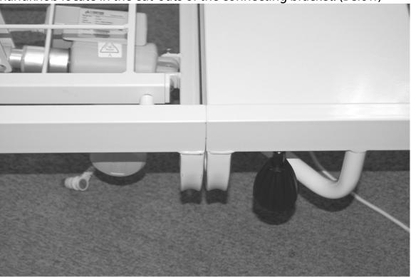
Connect the remaining motors and handset to the control box. Note the direction of the connectors. The hand control connection is on the side of the control box, the four motor connections are colour coded and labelled. (Below)
