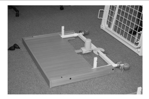
With the bed end on the floor, take either the head or foot frame and offer the two locating brackets on the bed-end into the frame as shown in the following sequence of images.
