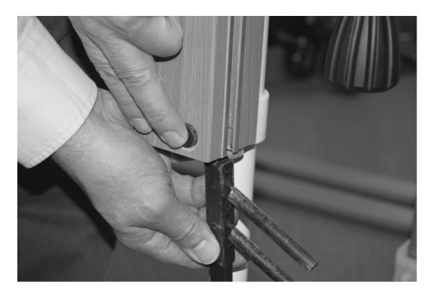
Fully insert the slider (pointed end up) until it locates in its lowest position. Fit both side rails to the slider with the rounded edge to the top. The other ends of the rails should rest on the floor. (see following images)
