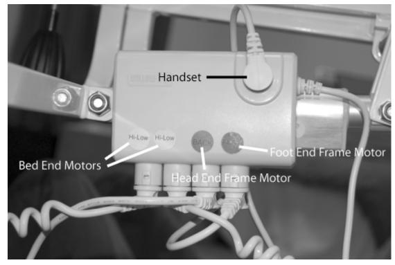
Connect the power supply to the mains and check the operation of the motors. If there is no function, check all connections are secure and the led is lit on the handset. Ensure the security key is plugged into the socket on the side of the handset. (see 'Operation' p.16)
