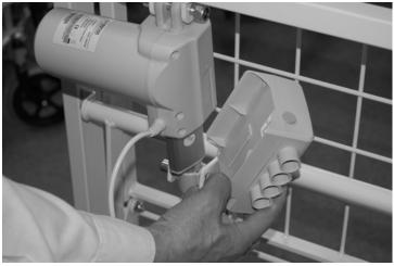
Plug the yellow banded bed-end motor into one of the sockets marked 'Hi-Low'.
