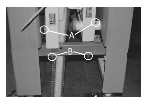
Using a 4mm allen key, fully undo the grub screws marked 'A' each side of the frames (keep these for later use). Carefully lift the frame up to clear the transportation bracket and manoeuvre it through the bedends and carefully place against a wall or on the floor. Repeat this for both frames.
